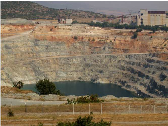
Fig. 3. Closed benching excavation.
